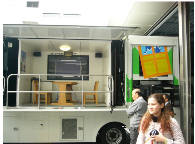
Figure 4. Earthquake simulation vehicle employed in Japan. This vehicle simulates the 1995 Kobe earthquake environment.
